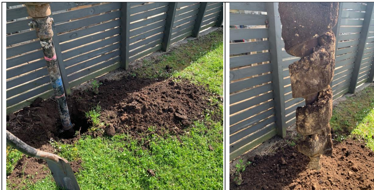
Figure 2 Images showing examples of auguring hole and retrieval of soil from depth.
