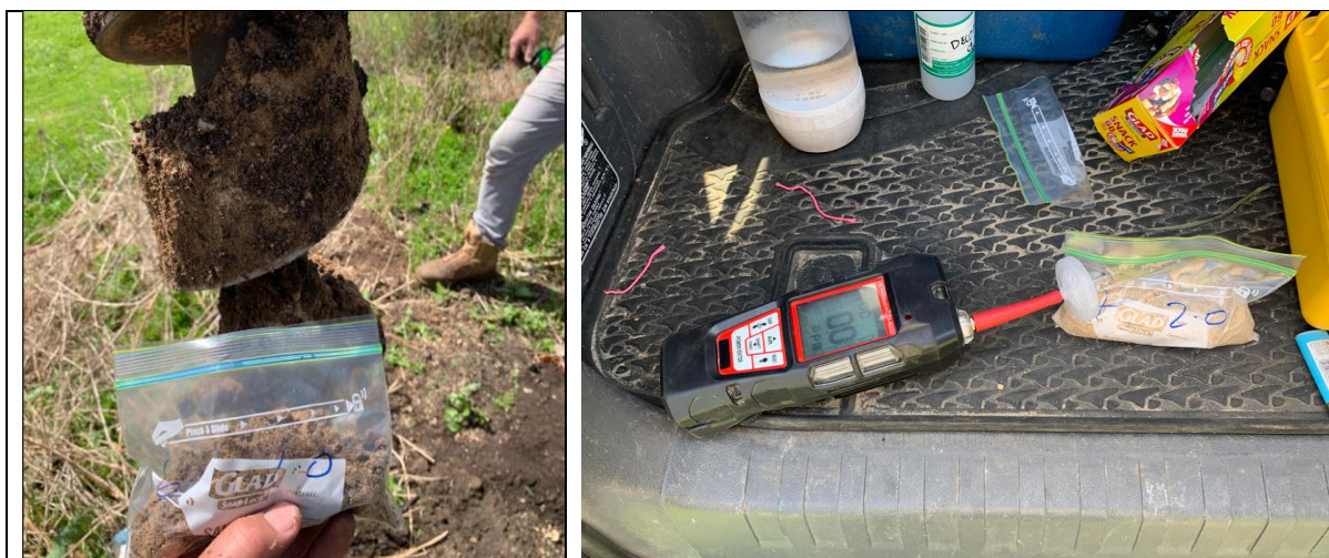
Figure 3 Images of samples being bagged for PID testing and PID testing the bag samples.
