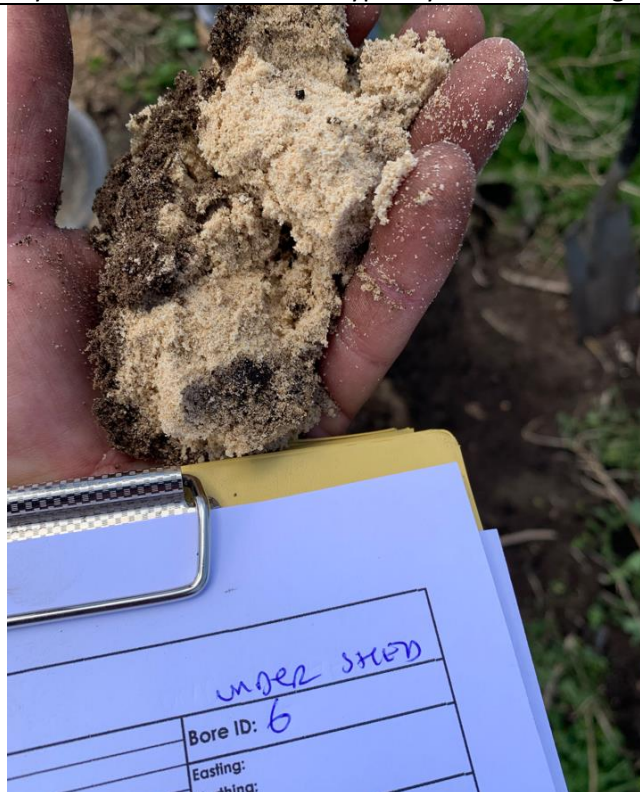
Image of the pale white yellow sand encountered typically in the 1-2 m bgl.
