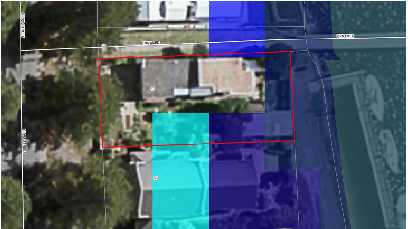
Figure 1: location of property with estimated 1% AEP flood depths, 2021 Moyne Planning Scheme Amendment C69 Flood Risk Mapping
