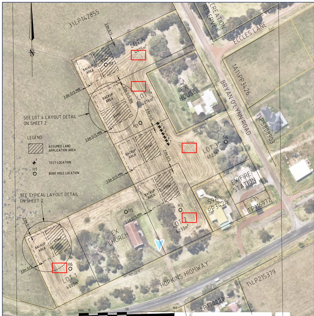
Figure 6 - Land capability plan with 10x15m rectangles (red) Base plan source: SITEC Engineering LCA Report
