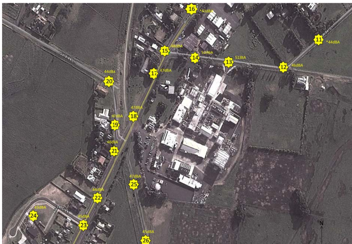
Figure 1 Aerial photo showing environmental noise measurement positions & level
