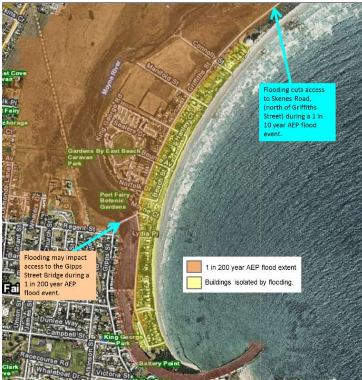
Figure 21. Griffiths Street residents isolated by flooding during a 1 in 200 year flood event.
