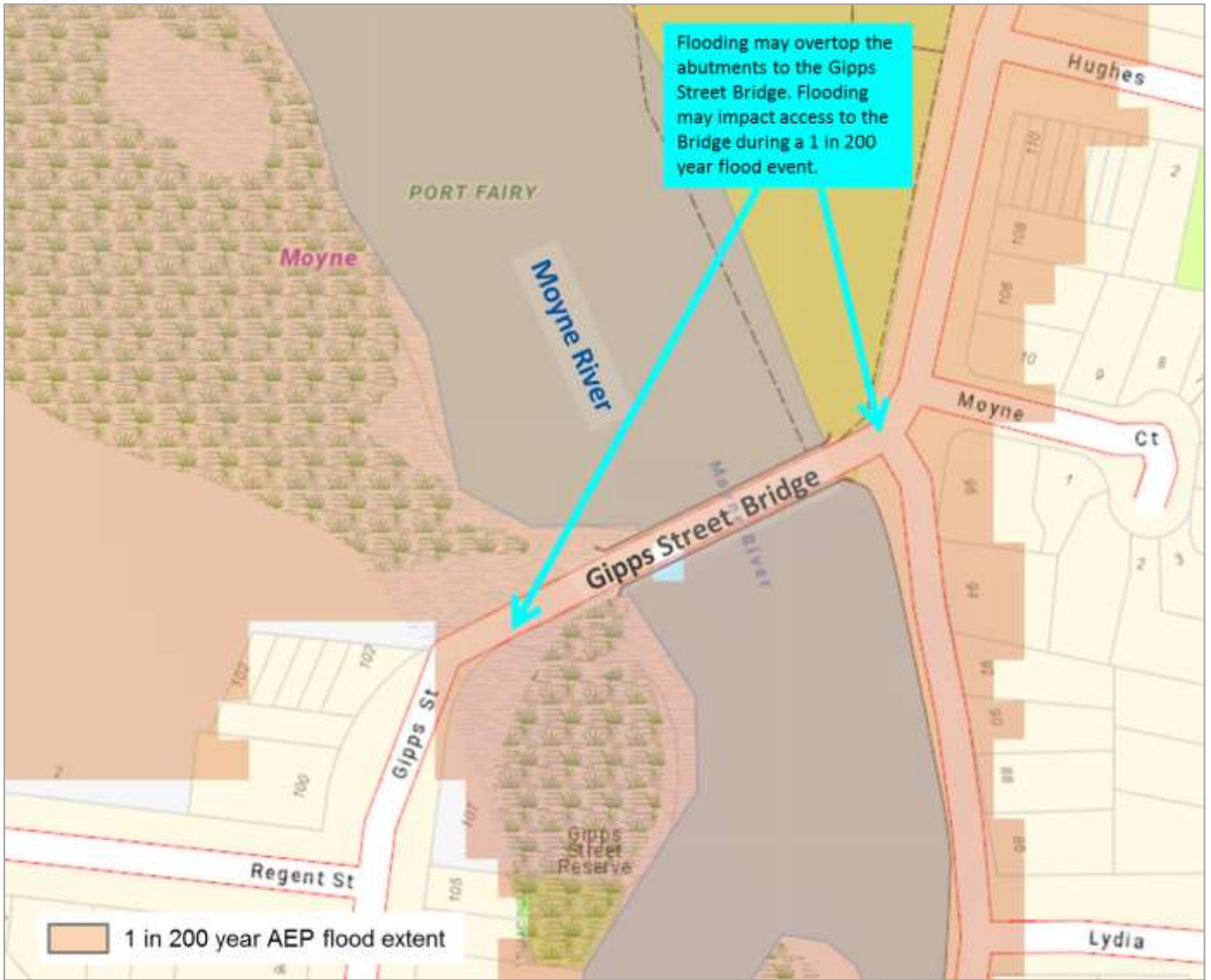
Figure 20. Flooding impacting the Gipps Street Bridge during a 1 in 200 year AEP flood event.
