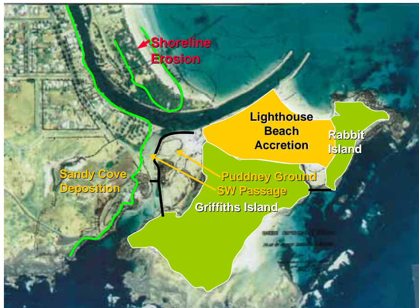
Figure 2-1 Original Shoreline and Sand Deposition Areas at Griffiths Island
