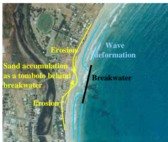
Figure 3-3 Typical Breakwater Behaviour
