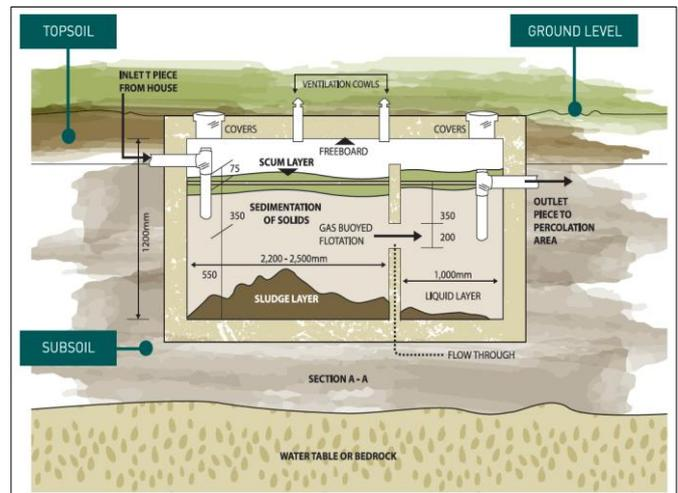
The scum helps prevent odours escaping and stops air entering. The treated effluent flows out of the tank through an outlet pipe as new wastewater enters.
