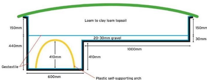
Figure 1 – WT & B system for primary treated effluent.
