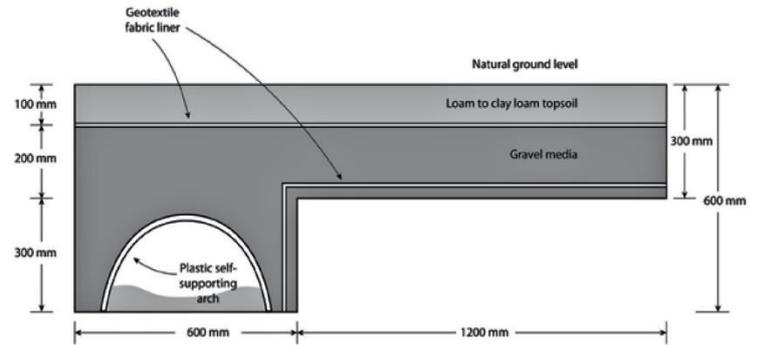
Figure 3 – WT & B cross-section (Source: Sydney Catchment Authority 2016).
