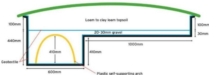
Figure 2 – WT & B system for secondary treated effluent. (Source: Vic EPA 2016)
