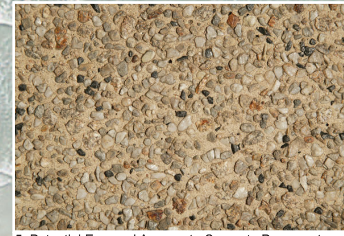
5. Potential Exposed Aggregate Concrete Pavement
