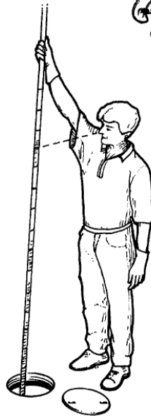
Checking sludge and scum levels in your septic tank.
